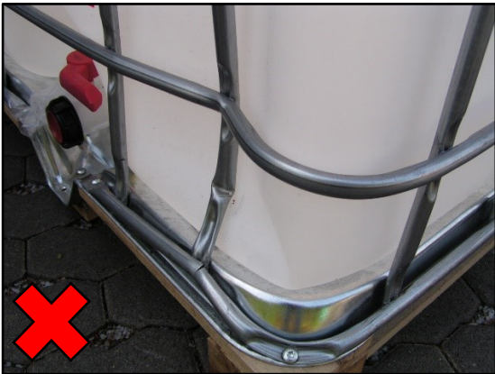
Frame is damaged
