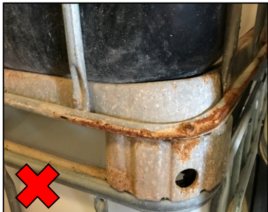
Corner foot is rusted
