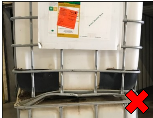
Frame is damaged
