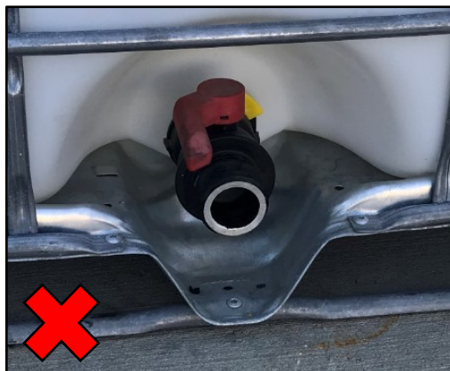
Valve left open upon delivery
