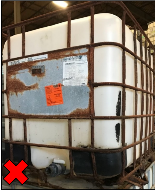
Entire frame of IBC is rusted
