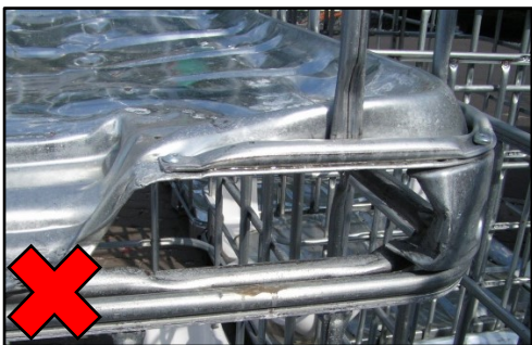
Corner foot is damaged
